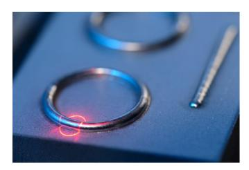
Image 1: Circulating measuring spot for inline measurements of LMD track heights. © Fraunhofer ILT, Aachen, Germany.
